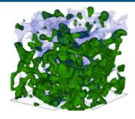
Mineral deposits formed from incompatibility between formation water and injected water impact fluid flow in reservoirs. Need to understand mechanism of deposit formation and design better inhibitors.
