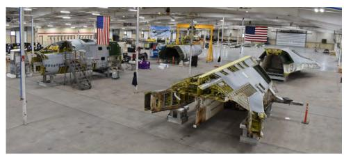
Supported by Dassault Systèmes' **Keep Them Operating** industry solution experience on the **3DEXPERIENCE** platform, NIAR will take the B-1 Lancer aircraft completely apart, scan every single structural element and digitally reassemble the aircraft to create virtual twins for future sustainment activities. The platform serves as the hub for visualizing, analyzing and predicting the aircrafts' performance.
